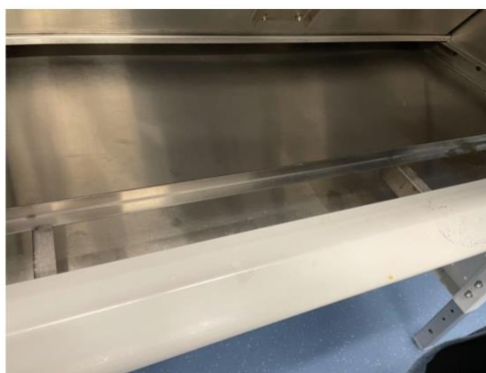
Figure 5- work surfaced propped up and front grille removed
