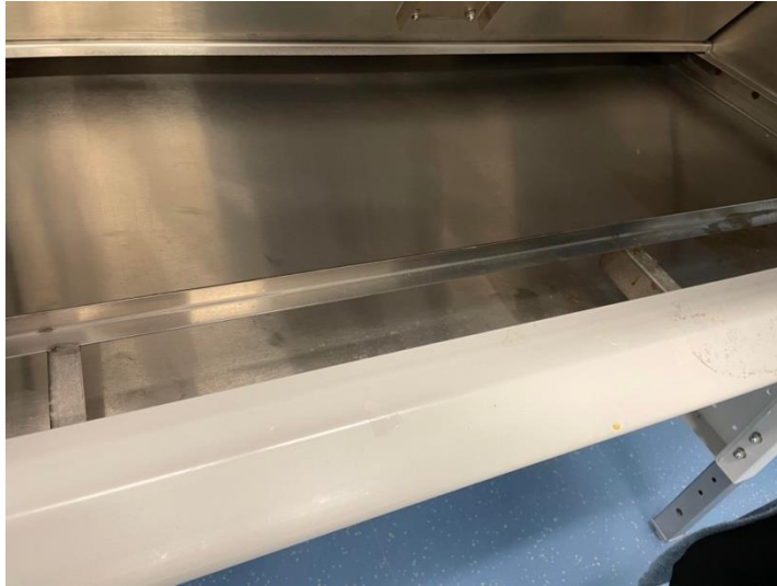
Figure 5- work surfaced propped up and front grille removed
